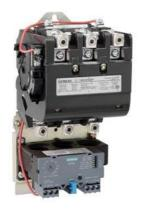
Non-reversing motor starter Size 3 1/2 Three phase full voltage Solid-state overload relay OLRelay amp range 50-200A 110-120/220-240VAC 60HZ coil Combination type No enclosure
