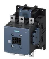
Power contactor, AC-3 300 A, 160 kW / 400 V AC (50-60 Hz) / DC operation 23-26 V AC/DC Auxiliary contacts 2 NO + 2 NC 3-pole, Size S10 Busbar connections Drive: conventional screw terminal NEMA version
