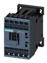
power contactor, AC-3 7 A, 3 kW / 400 V 1 NC, 24 V DC 0.7-1.25\* US, with diode integrated, 3-pole, size S00, spring-type terminal suitable for PLC outputs not expandable with auxiliary switch
