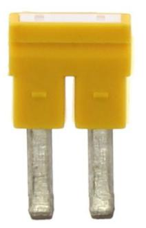
Insulated cross-connector, No. of poles: 2, Mounting type: Plug in, Width: 12.1 mm, Colour: Yellow
