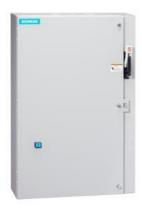
Non-reversing motor starter, Size 2 1/2, Three phase full voltage, Solidstate overload relay, OLR amp range 25-100A, Combination type, 100A non-fusible disconnect, Enclosure NEMA type 1, Indoor general purpose use, Extra-wide enclosure
