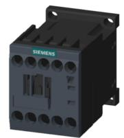
Power contactor, AC-3 9 A, 4 kW / 400 V 1 NC, 220 V AC, 50 / 60 Hz 3-pole, Size S00 screw terminal
