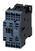
power contactor, AC-3 17 A, 7.5 kW / 400 V 1 NO + 1 NC, 24 V DC communication-capable, 3-pole, Size S0, Spring-type terminal
