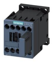
power contactor, AC-3 7 A, 3 kW / 400 V 1 NO, 24 V DC 0.85-1.85\* US, with varistor plugged on, 3-pole, size S00, screw terminal not expandable with auxiliary switch
