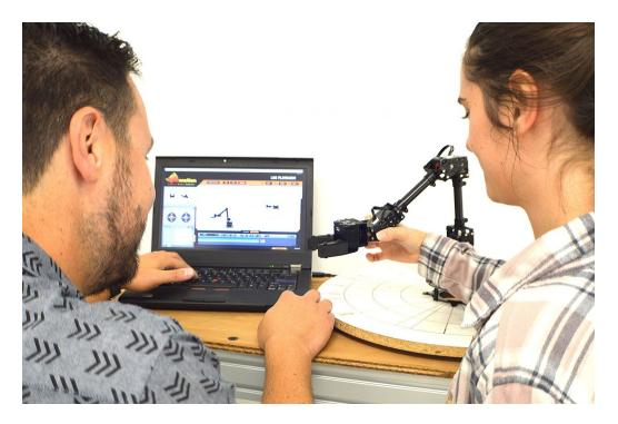
Given that the structure of the arm is comprised of modular brackets and servos, purpose-built and ultralight aesthetic plastic shells give a futuristic look to the arm without impeding any motion. The shells are held in place using neodymium magnets, and vinyl stickers allow for personnalisation.
