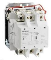
Mechanically held lighting contactor, Contactor amp rating 200A, 0 N.C. / 2 N.O. poles, 440VAC 50HZ/480VAC 60HZ coil, Non-combination type, Enclosure NEMA type (open), No enclosure
