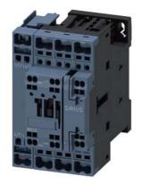
Contactor, AC-1, 35 A/400 V/40  $^{\circ}$ C, S0, 4-pole, 110 V AC/50 Hz, 120 V/60 Hz, 1 NO+1 NC, Spring-type terminal
