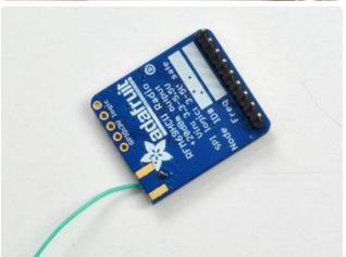
Strip a mm or two off the end of the wire, tin and solder into the ANT pad.
