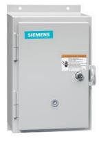
Reversing motor starter, Size 0, Three phase full voltage, Solid-state overload relay, OLR amp range 3-12A, Non-combination type, Enclosure type 12, Dust/drip proof for indoors, Standard width enclosure
