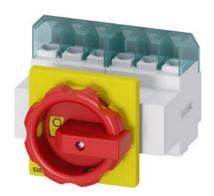
SENTRON, Switch disconnector 3LD, emergency switching-off switch, 6-pole, lu: 25 A, operating power / at AC-23 A 400 V: 9.5 kW, front-mounted, rotary operating mechanism, Red / yellow, 4-hole mounting of the handle
