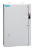
Non-reversing motor starter, Size 1 3/4, Three phase full voltage, Solid-state overload relay, OLR amp range 10-40A, Combination type, 60A non-fusible disconnect, Enclosure NEMA type 4/12, Water/dust tight for outdoors, Extra-wide enclosure
