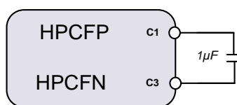
Figure 41: Charge Pump Flying Capacitor
