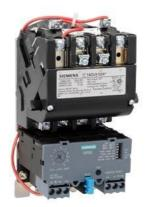
Non-reversing motor starter Size 2 Three phase full voltage Solid-state overload relay OLRelay amp range 13-52a 208VAC 60HZ coil Combination type No enclosure
