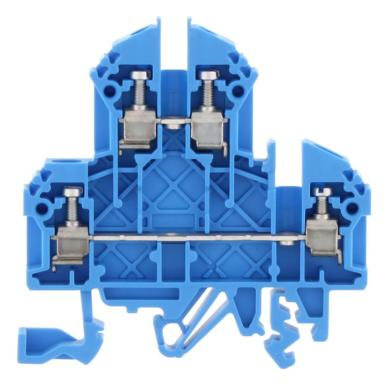
Double-level terminal, Screw connection, Mounting type:Mounting rail TS 35/7.5 and TS 32, Rated cross-section: 2.5 mm<sup>2</sup>, Width: 5 mm, Colour: Blue
