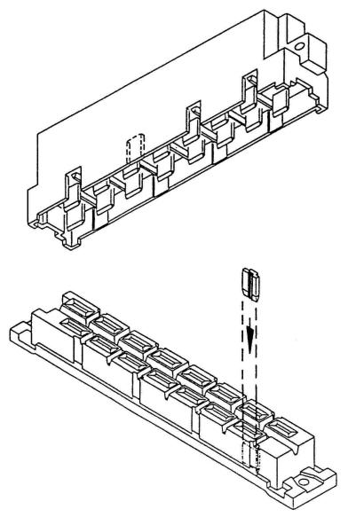
To avoid cross-plugging of adjacent connectors a coding system is required. Insert the code key 09 06 001 9918 into one of the keyways of the female connector as shown in the drawing. Break out the corresponding area of the male shroud. Connectors coded this way can only be applied in a minimum rack spacing of 20.32 mm.
