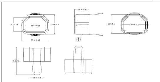
Warning: When removing connector with this sleeve included, take care not to damage the inlet when removing the connector. To remove the Sleeve that remains in the inlet after cord extraction, ensure the power cord is not plugged into power and use a non-conductive tool to extract.
