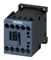
power contactor, AC-3 12 A, 5.5 kW / 400 V 1 NO, 24 V DC 3-pole, Size S00 screw terminal
