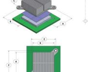
1) Dimension A is the length of the heat sink in the direction of the flow.
