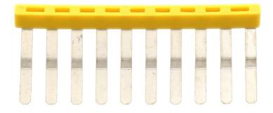
External insulated cross-connector, No. of poles: 10, Mounting type: Plug in, Width: 50.1 mm, Rated current: 27 A; Colour: Yellow
