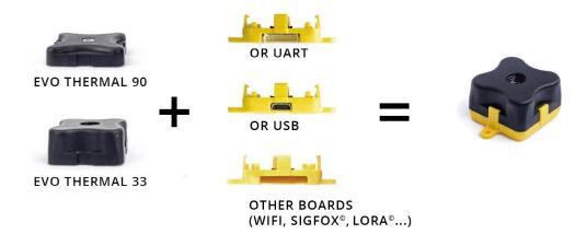
Evo Thermal sensors consist of a thermographic sensing device (black module, 7g or 9g) and a choice of backboard (yellow module, 3g), which simply plugs-in to provide the sensor with a communication link and power management capabilities. You simply choose the backboard that best suits your application and communication protocol!
