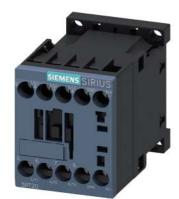
power contactor, AC-3 12 A, 5.5 kW / 400 V 1 NC, 24 V DC 0.7-1.25\*US with integrated suppressor diode 3-pole, size S00 screw terminal suitable for PLC outputs not expandable with auxiliary switch
