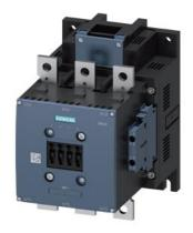
power contactor, AC-3 265 A, 132 kW / 400 V AC (50-60 Hz) / DC operation 23-26 V AC/DC auxiliary contacts 2 NO + 2 NC 3-pole, frame size S10 busbar connections drive: conventional screw terminal
