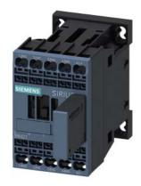
Coupling contactor relay, 3 NO + 1 NC, 24 V DC, 0.85  $\dots$  1.85\* US, with varistor plugged on, Size S00, Spring-type terminal
