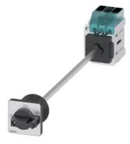
Load disconnector 3LD3, lu 16 A Main switch 3-pole Rated operating capacity at AC-23 A at 400V 7.5kW floor mounting Basic switch with door coupling Central hole mounting 22.5mm Toggle drive black 48x48 mm with auxiliary switch 1OE + 1S
