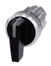
Illuminable selector switch, 22 mm, round, metal shiny, black, Selector switch long, 3 switch positions I-O-II, latching, actuating angle  $2x45^\circ,\,10:\!30h/12h/13:\!30h$
