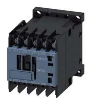
power contactor, AC-3 12 A, 5.5 kW / 400 V 1 NC, 24 V DC 0.7-1.25\* US, with suppressor diode integrated 3-pole, size S00 ring cable lug connection suitable for PLC outputs not expandable with auxiliary switch
