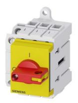
Load disconnector 3LD3, lu 63 A Main switch 3-pole Rated operating capacity at AC-23 A at 400V 22.0 kW Installation in distribution boards, Basic switch with selector knob red / yellow with auxiliary switch 1OE + 1S
