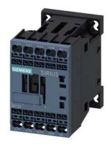
power contactor, AC-3 12 A, 5.5 kW / 400 V 1 NC, 42 V AC, 50 / 60 Hz 3-pole, Size S00 Spring-type terminal
