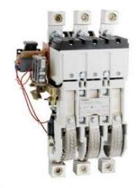
Mechanically held lighting contactor, Contactor amp rating 300A, 0 N.C. / 3 N.O. poles, 110VAC 50HZ/120VAC 60HZ coil, Non-combination type, Enclosure NEMA type (open), No enclosure
