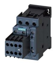
power contactor, AC-3 25 A, 11 kW / 400 V 2 NO + 2 NC, 110 V AC/50 Hz Hz 120 V/60 Hz 3-pole, Size S0 screw terminal Removable auxiliary switch
