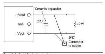
Output ripple and noise test setup
