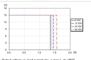
Output voltage vs. load current at  $I_0$  > max  $I_0$  at +25°C. (Balance Load)
