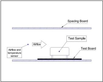
For products with base plate used in a sealed box application. Cooling is achieved mainly by airflowing. The Output Current Derating graphs are found in the Output section for each model. The product is tested in a sealed box test set up with ambient temperatures 25°C.
