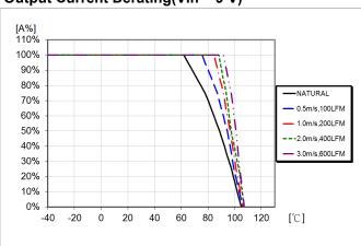
Available load current vs. ambient air temperature and airflow at  $V_{\rm I}$  = 9 V. See Thermal Consideration section.
