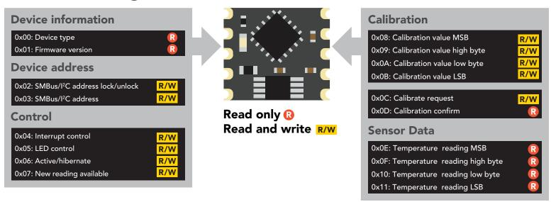
The default device address is **0x68** This address can be changed.
