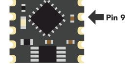
The Interrupt control register adjusts the function of pin 9 (the interrupt output pin).
