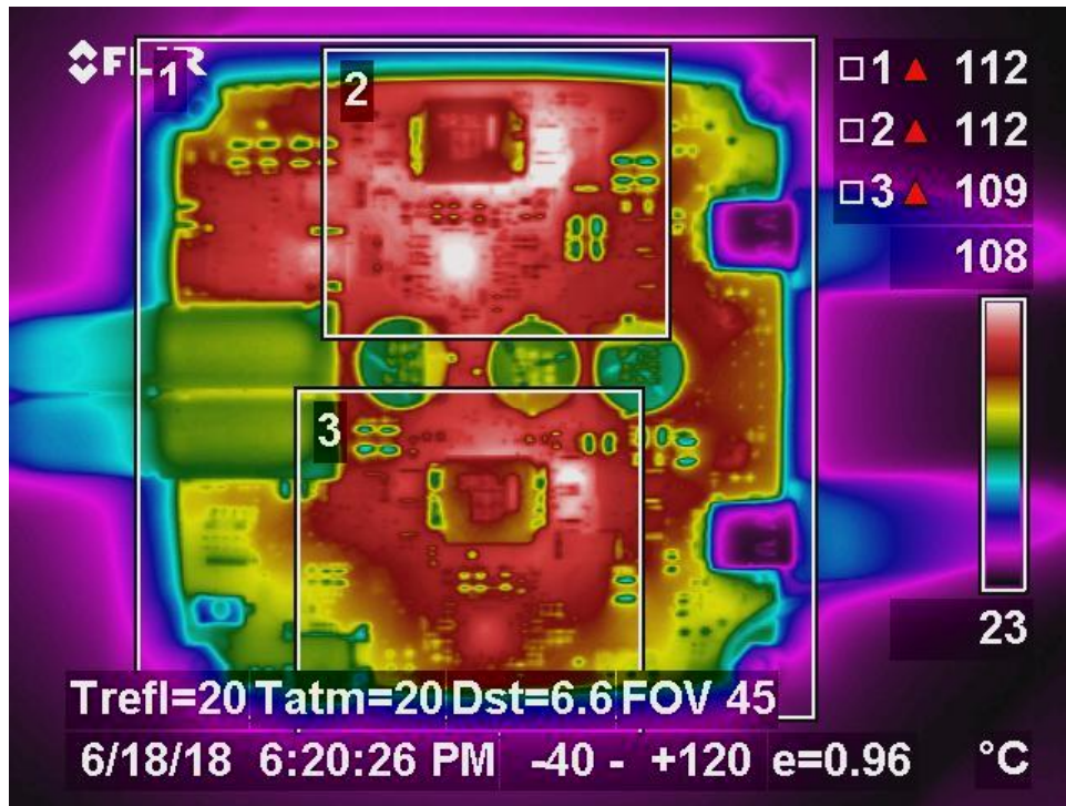
Figure 11 - Dual Port: 13.5 Vin, 20 Vout at 5 A each port (200 W total)
