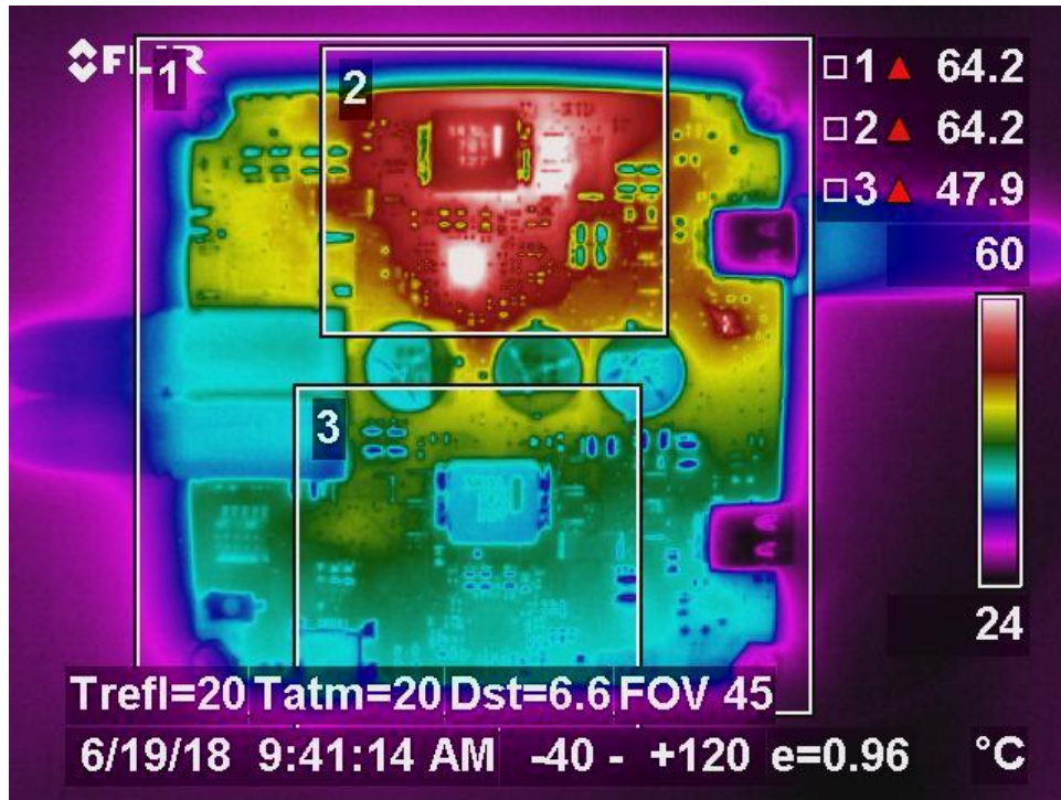
Figure 8 - Single Port: 13.5 Vin, 20 Vout at 3 A (60 W total)
