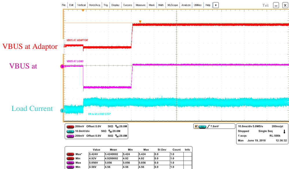
Figure 6 – 0.2A to 3A Load Step Event Resulting in 400mV VBUS Bias to Account for Cable Drop
