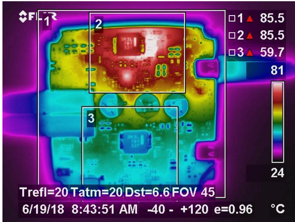
Figure 10 - Single Port: 13.5 Vin, 20 Vout at 5 A (100 W total)
