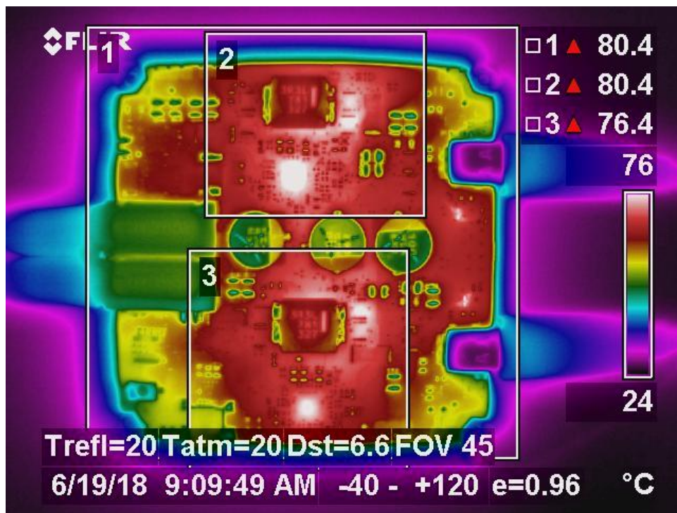
Figure 9 - Dual Port: 13.5 Vin, 20 Vout at 3 A each port (120 W total)
