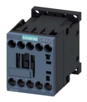
power contactor, AC-3 7 A, 3 kW / 400 V 1 NO, 24 V DC 0.85-1.85\* US, with diode integrated, 3-pole, size S00, screw terminal not expandable with auxiliary switch
