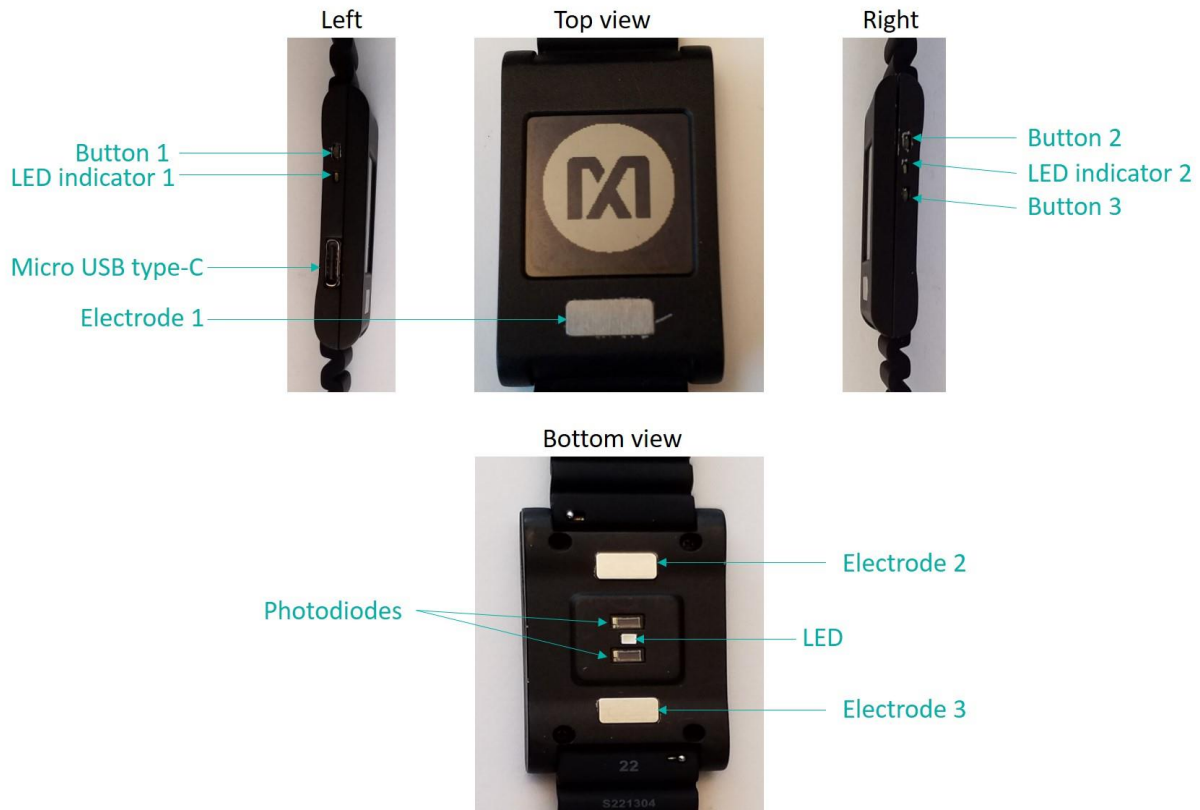
Figure 1. MAXREFDES101# wearable form factor in detail.
