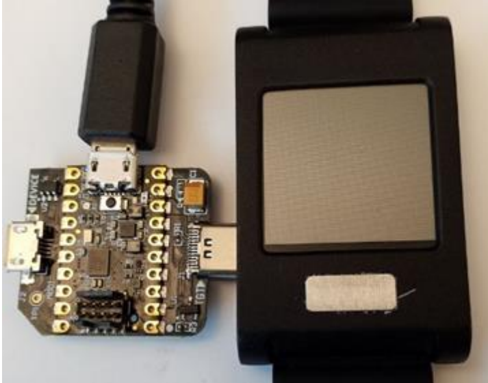
Figure 10. Pico adaptor board connected through micro USB Type-C.
