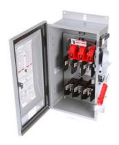
Siemens Low Voltage Circuit Protection Heavy Duty Safety Switches. Type: ENCLOSED, SAFETY SWITCH Std: UL V. Rating: 240V A. Rating: 200A Wattage: 3W No. Of Poles: 3P F. Rating: 60Hz Action: SINGLE THROW Material: 304SS Enclosure: TYPE 12. 2-3 point mounting holes. Insulation: YES O. Cycles: 8000 O. Temperature: (-20F-120F) AMBIENT TEMPERATURE Environmental Conditions: INDUSTRIAL
