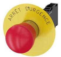
EMERGENCY STOP mushroom pushbutton, 22 mm, round, metal, shiny, red, 40 mm, positive latching, acc. to EN ISO 13850, pull-to-unlatch mechanism, with yellow backing plate, inscription: Arrêt d'urgence, with holder, 1 NO+1 NC, screw terminal
