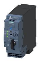
SIRIUS Compact load feeder DOL starter for IO-Link 690 V 24 V DC 3...12 A IP20 Connection main circuit: plug-in, without terminals Connection control circuit: Spring-type terminal
