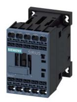
Coupling contactor relay railway 2 NO + 2 NC, 110 V DC, 0.7 ... 1.25\* US, with varistor integrated, Size S00, Spring-type terminal
