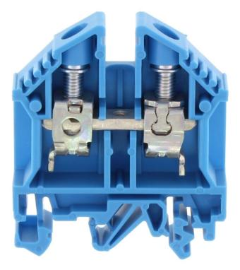
Feed-through terminal, Screw connection, Mounting type:Mounting rail TS 35/7.5 and TS 32, Rated cross-section: 16 mm<sup>2</sup>, Width: 12 mm, Colour: Blue
