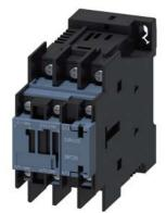
power contactor, AC-3 25 A, 11 kW / 400 V 1 NO + 1 NC 24 V DC, with integrated diode combination, 3-pole, Size S0 ring cable lug connection
