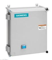
Non-reversing motor starter, Size 3 1/2, Three phase full voltage, Amb. compensate bimetal OLR, Contactor amp rating 115A, 240V 50Hz / 277V 60Hz coil, Non-combination type, Enclosure type 4X fiberglass, Water/dust tight noncorrosive
