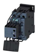
Capacitor contactor, AC-6b 16.7 kVAr, / 400 V 1 NO + 2 NC, 24 V AC, 50/60 Hz 3-pole, Size S0 screw terminal
