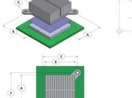
1) Dimension A is the length of the heat sink in the direction of the flow.
