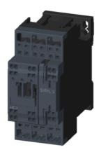
power contactor, AC-3 25 A, 11 kW / 400 V 1 NO + 1 NC, 208 V AC 50/60 Hz 3-pole, Size S0 Spring-type terminal
