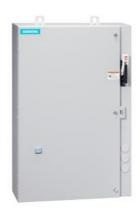
Non-reversing motor starter, Size 1, Three phase full voltage, Solid-state overload relay, OLR amp range 0.75-3.4A, 240V 50Hz / 277V 60Hz coil, Combination type, 30A non-fusible disconnect, Encl NEMA type 4X 304 S-Steel, Water/dust tight noncorrosive, Extra-wide enclosure
